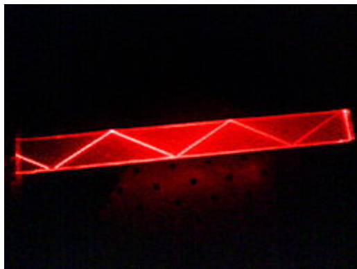
Figure 2: Total internal reflection in a block of Plexiglas surrounded by air using a laser as a source.
